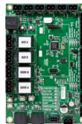
P/N 720-100105 EN-ACM—2-door add-on expansion module
